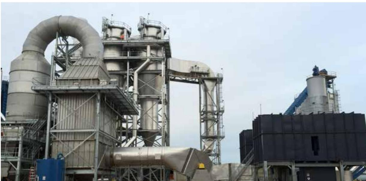
*Wet electrostatic precipitator*
